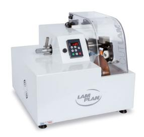
Equipped with an independent decanting/ recirculation tank, you can easily make slow cuts in optimum conditions of cooling.
